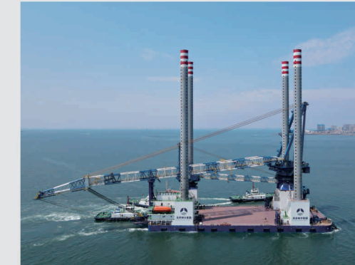
（华夏金租神大01/02）1200T风电安装平台(主吊机1200t;4-5000T液压插销升降系统) (Huaxia Financial Leasing Co., Ltd Shenda 01/02)1200T Wind Power Installation Platform (Main Crane 1200t; 4-5000T hydraulic pin lifting system)
