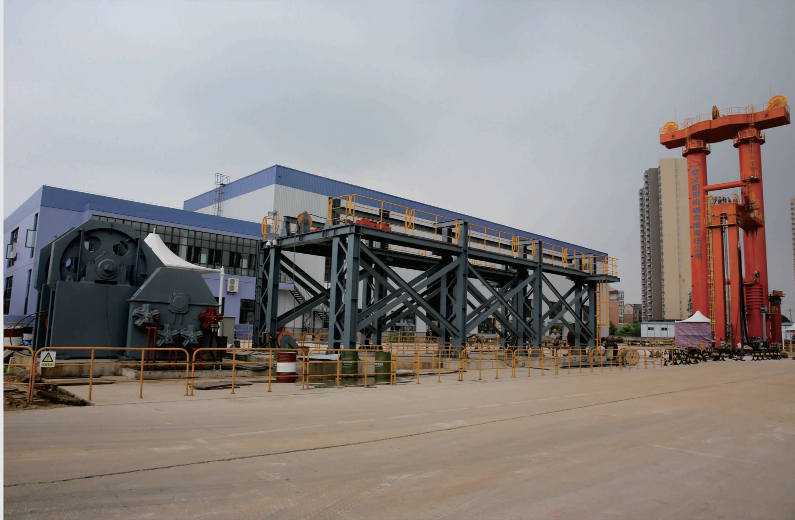
甲板锚作/定位系统试验系统(塔架动载300吨，有效行程320m) Deck anchoring operation/positioning system test system(Tower dynamic load 300t, effective travel 320m)
