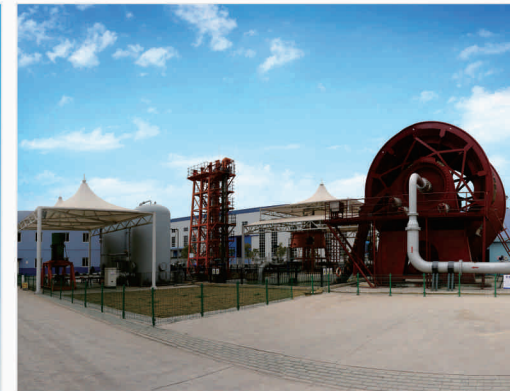
6000m 3 /h液货装卸与外输系统试验台 6000m 3 /h test bench oil liquid cargohandling system
