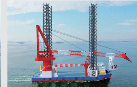
天津港航1800T风电安装船（吊机1800t、380t；4-9000T电动齿轮齿条升降系统） Tianjin Port and Waterway Engineering Co.,Ltd 1800T wind power installation ship (crane 1800t, 380t; 4-9000T electric gear rack lifting system)
