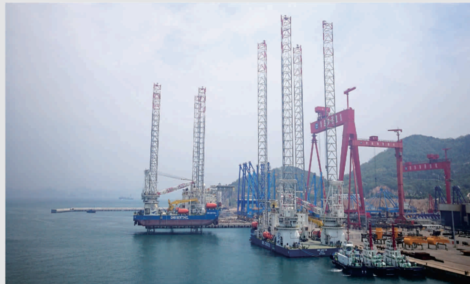
SE350LB自升式海工辅助平台(110m桁架式桩腿、最大工作水深80m) SE350LB Self elevating Marine Auxiliary Platform(110m truss type pile legs, maximum working water depth 80m)
