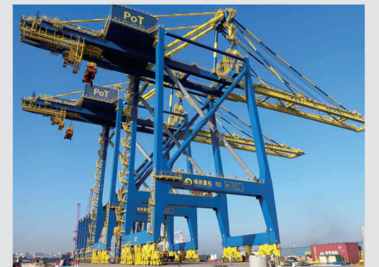
65T-63M集装箱岸桥 65T-63M Ship-to-Shore Container Gantry Crane
