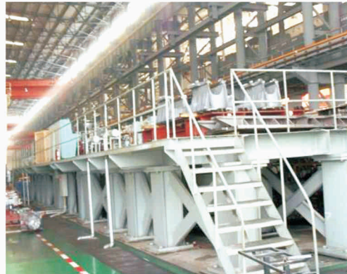
2×300T*m舵机负载试验台 2×300T*m load test bench for the steering gear
