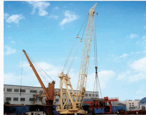
15000T*m起吊设备负载试验台 15000T*m load test bench for the lifting appliance
