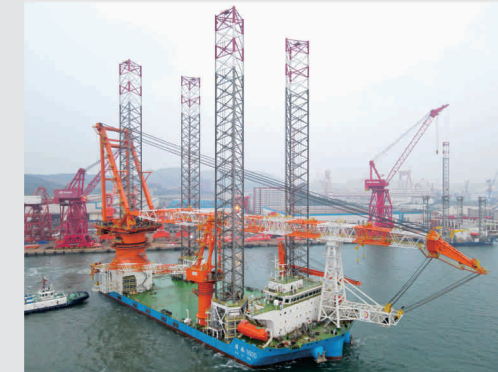
华西海工1600T风电安装平台（4-8820T电动齿轮齿条升降系统、主吊机1600t） Huaxi Offshore 1600T Wind Power Installation Platform (4-8820T Electric Gear and Rack Lifting System, Main Crane 1600t)
