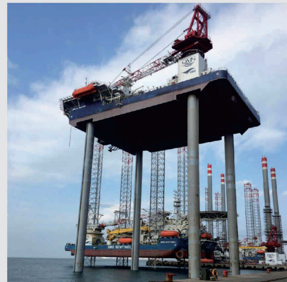
SE-300LB自升式海工平台（91m圆柱桩腿、最大工作水深60m） SE-300LB Self elevating Offshore Platform(91m cylindrical pile leg, maximum working water depth 60m)
