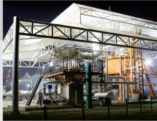
3000kW透平货油泵负载试验台 3000kW test bench for turbine cargo oil pump load
